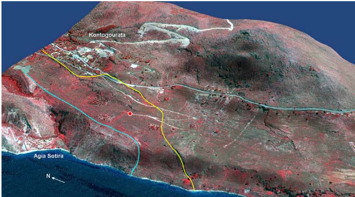
Figure 5: Location of trial borehole showing diagnosed channel route The borehole is surrounded by solid limestone bedrock on the west and east
