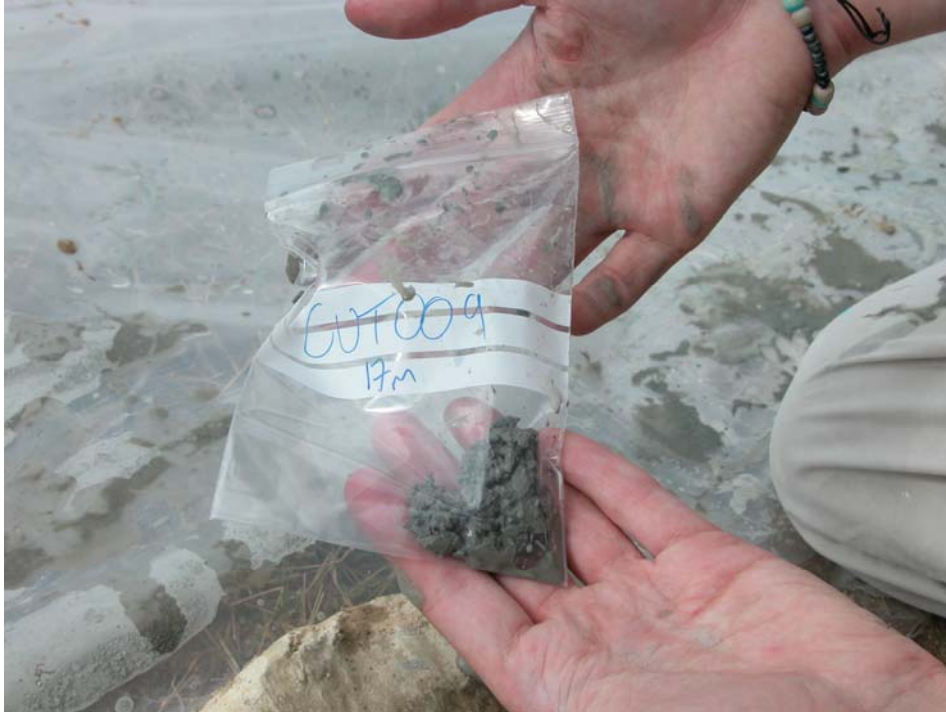
Figure 6: Borehole sample captured from drill cuttings The samples have been analysed at the Bulgarian Academy of Sciences
