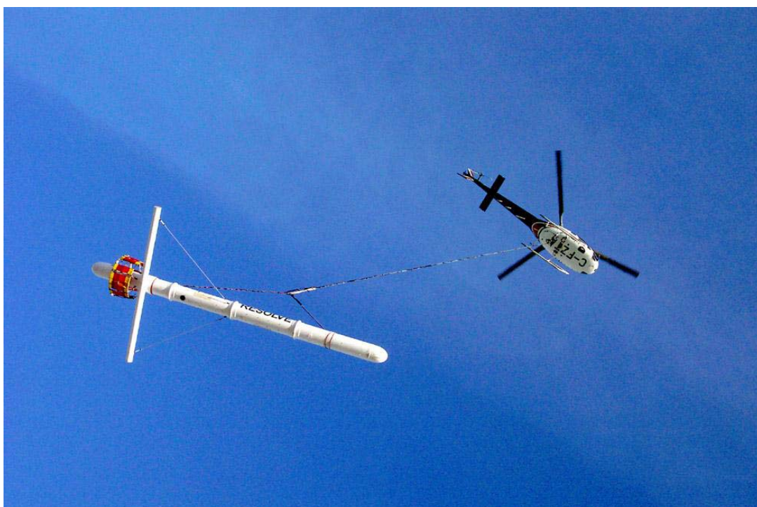
Fugro RESOLVE airborne electromagnetic survey system
