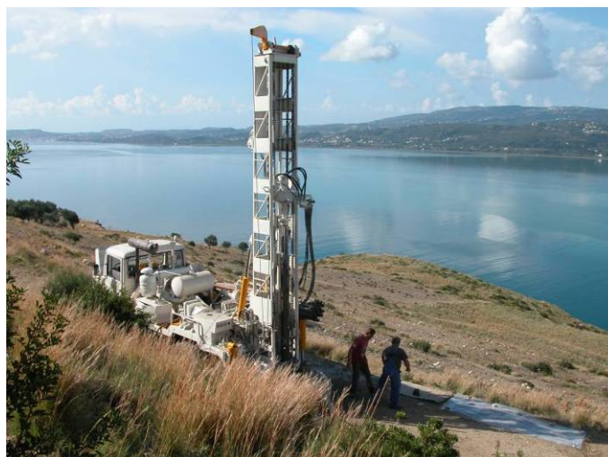
Figure 2: Drilling a 122 metre (400 foot) test borehole in October 2006 No solid limestone bedrock was encountered between the surface and sea level
